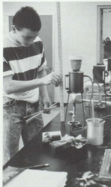
Pat Brown, 12, measures the specific heat of lead shot in boiling water. (M.A.)
