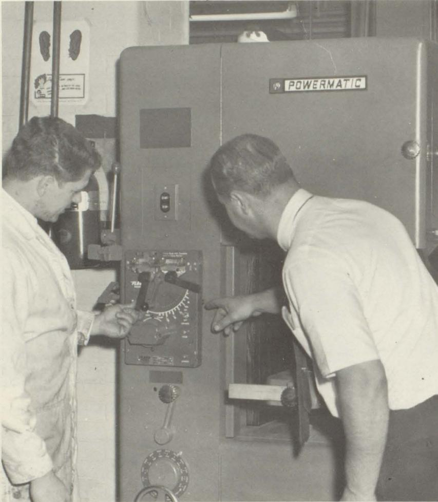
Mr. Rayshich explains the blade welder on the automatic bandsaw to Andy Daulton.
