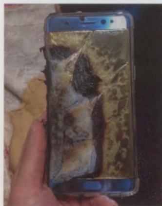
◀ Samsung’s newest Android smartphone, the **Galaxy Note7**, was discontinued after less than two months when it was discovered that battery defects led to excessive heat, causing fires and even explosions.
