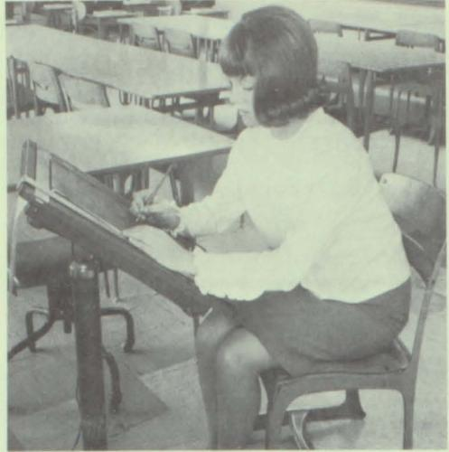
The mimeoscope, an illuminated drawing board, is used for preparing pictures in Gazette.
